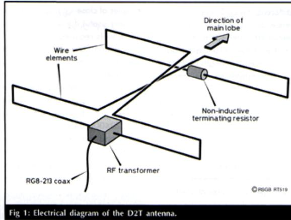
Fig 1: Electrical diagram of the D2T antenna.
